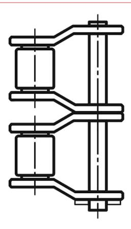
For chain size =  $1 \frac{1}{2} \times 1$ For chain type = 24 B-2
